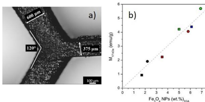
Figure 1: a) Detail of the 3D printed hexagons; b) evolution of magnetization (at  $H = 17$  kOe) values for the 3D printed magnetic polymers (75Eb25BA squares and 50Eb50BA circles) as a function of  $\text{Fe}_3\text{O}_4$  nanoparticles concentration estimated by TGA measurements (dotted line is a guide to the eyes).
