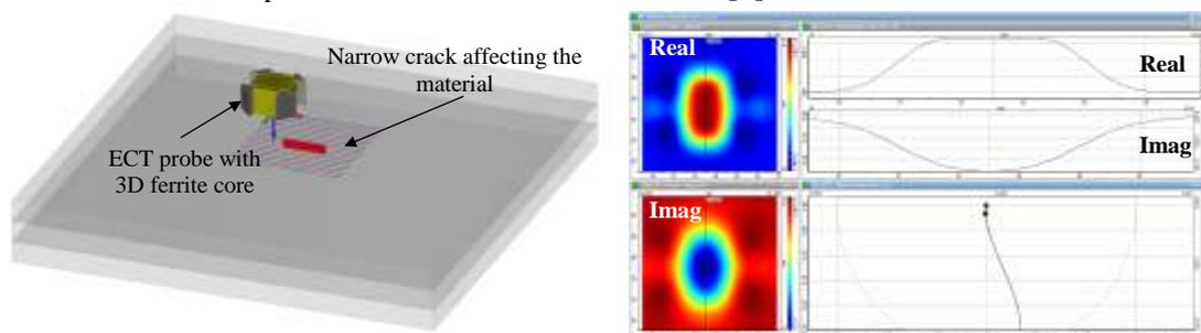
Figure 1: Simulation of an ECT inspection by means of a coupled approach. A 2D map of the complex impedance change of the probe due to the flaw is computed at a single frequency.
