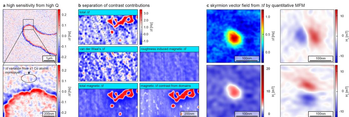
Figure 1: a) MFM data of a Pt(10nm)/Co(0.6nm)/Pt(3nm) trilayer recorded with a cantilever with  $Q = 1'000'000$ . b) Separation of MFM contrast contributions required to make sub-10nm skyrmions visible. c) MFM data of an isolated skyrmion in a  $[\text{Ir}(1\text{nm})/\text{Co}(0.6\text{nm})/\text{Pt}(1\text{nm})]_{\times 5}$ -multilayer with all vector components of the field obtained by quantitative MFM techniques.
