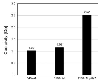
Figure 2: Relationships between coercivity and wet synthesis conditions.
