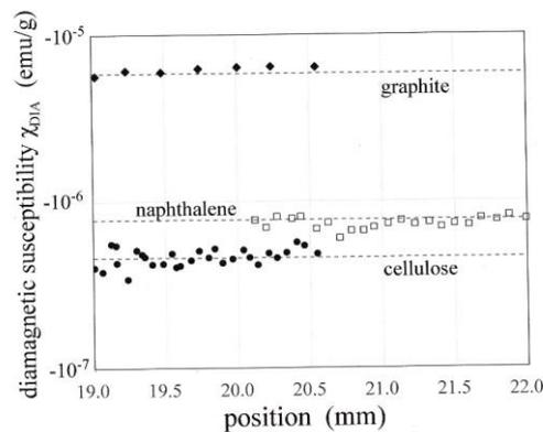
Fig. 1 Experimental  $\chi_{\text{DIA}}$  values of a single particle obtained at different positions during its field-induced translation. Equation (1) is used in calculating  $\chi_{\text{DIA}}$ .
