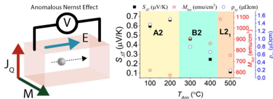
Figure 1: Figure 1: Left: Schematic of the ANE. Right: Dependence of ANE, magnetisation and anomalous Hall resistivity on the ordering of Co<sub>2</sub>MnSi thin films.
