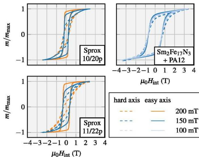
Figure 1. Hysteresis loops in hard and easy axes of three samples measured with the VSM, where  $H_{int}$  is the internal field, considering a demagnetization factor of  $N = 1/3$ . The samples are aligned with different magnitudes of the external field [4].
