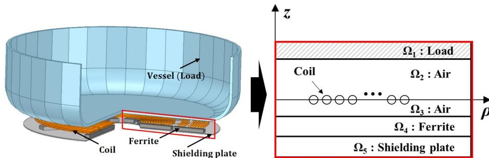
Figure 1: Schematic diagram of domestic induction cooker and an axisymmetric model for the analytical formulation of induction heating problem
