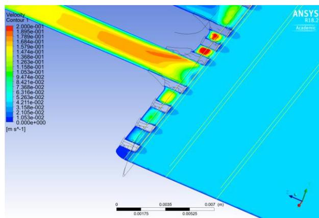
Figure 1: FLUENT simulation of the flow distribution at the inlet of the regenerator.
