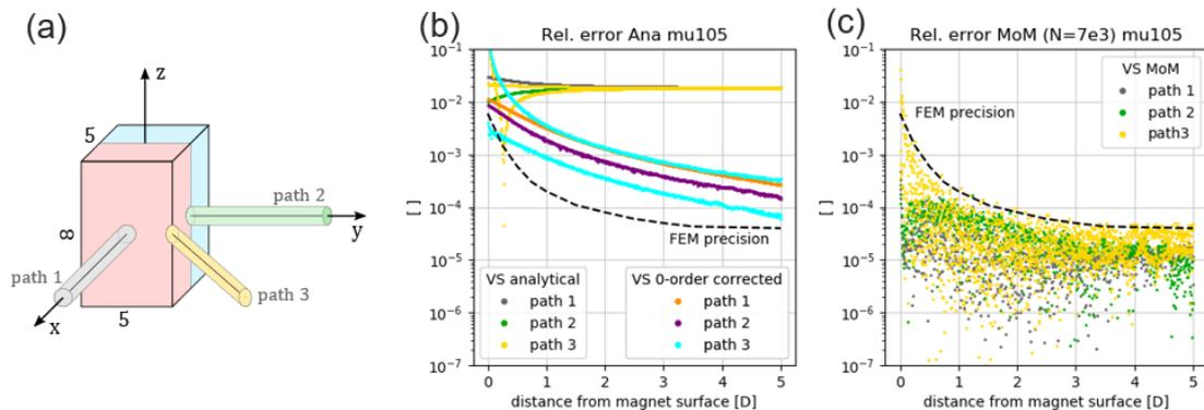
Figure: (a) Sketch of magnet and paths where field is tested. (b) Relative error of analytical models. (c) A method of moments with less than  $10^4$  cells undercuts a FEM with more than  $10^6$  elements and computes several orders of magnitude faster.
