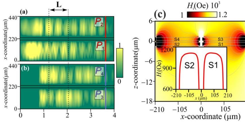
Figure 1: Maps of component  $m_z$  of dynamic magnetization in bottom layer (a), top layer (b); distribution of the internal magnetic field  $H_i$  (inset:  $H_{ix}$  profile for the lateral system of the bottom layer)(c)
