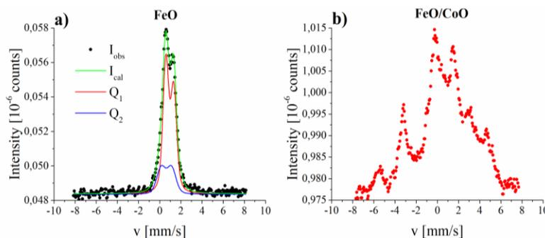
Figure 1: CEMS measurements of FeO (black points) in MgO/FeO/MgO (a) and MgO/FeO/CoO (b).
