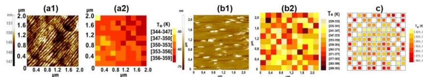
Figure 1: a1), a2) : Topography scan and  $T_M$  distribution map for a  $2 \times 2 \mu\text{m}$  of 400 nm film, respectively; b1), b2) : Topography scan and  $T_M$  distribution map for a  $2.2 \times 2.2 \mu\text{m}$  of 100 nm film, respectively; c)  $2.2 \times 2.2 \mu\text{m}$  area of 100 nm film.
