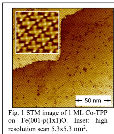
Fig. 1 STM image of 1 ML Co-TPP on Fe(001)-*p*(1x1)O. Inset: high resolution scan 5.3x5.3 nm<sup>2</sup>.
