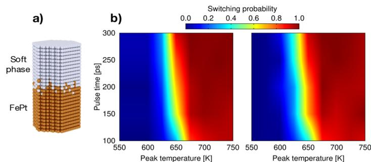
Figure 1: (a) Atomic structure of the investigated grain composed of FePt (gold) and Soft phase (silver) showing the intermixing. (b) Comparison of switching probability as function of pulse time and peak temperature for zero (left) and small intermixing (right).
