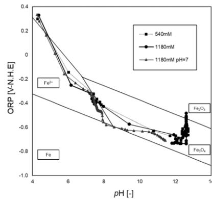
Figure 1: pH - ORP diagram with nano-ferrite fabrication.
