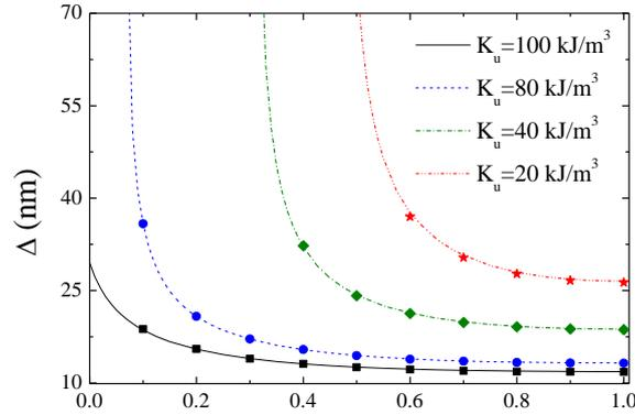
Figure 1: Domain wall size as a function of the two sublattice saturation magnetization ratio. Dots are micromagnetic simulations and lines one dimensional approximation.
