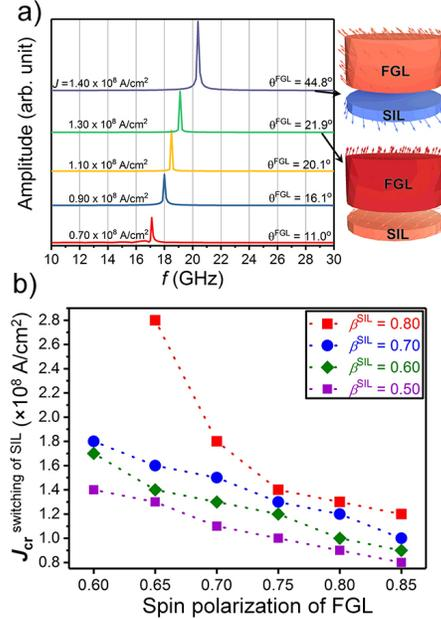
**Figure 1:** (a) RF spectra calculated from  $M_x$  oscillation of FGL for  $\beta^{SIL} = 0.80$  and  $\beta^{FGL} = 0.75$  for different  $J$ . The oscillation cone angle of FGL is also shown. (b) Critical current density required for the magnetization switching of SIL as a function of  $\beta^{FGL}$  and  $\beta^{SIL}$  in all-in-plane STO.
