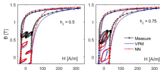
Figure 1: Hysteresis cycles obtained by a fundamental plus the 3<sup>rd</sup> order harmonic of B: measured curves are compared with those simulated by either the Preisach model (VPM) or the Neural Network (NN) for two different values of the harmonic ratio  $h_r$ .
