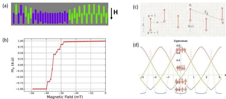
Figure 2. (a) Schematic of a structure with a periodic modulation and (b) its hysteretic behavior calculated using (b) micromagnetic simulations. (c) Schem featuring the dumbbell model used to characterize the energetics of the system and (d) the resulting energy bands of the possible magnetic states of a modulated chain of dumbbells.
