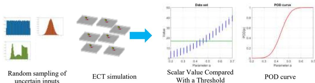
Figure 2: Typical model based approach for performance demonstration of a NDT method using Probability of Detection (POD) curves.
