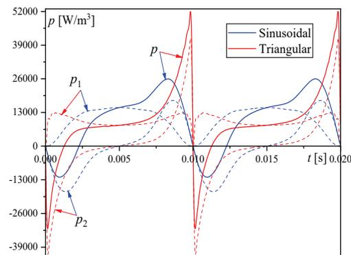
Figure 1: Instantaneous magnetising power and its components.
