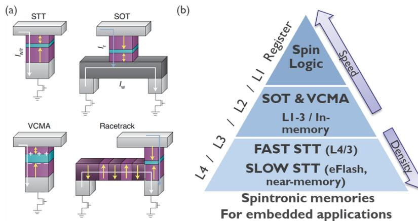
**Figure:** (a) Various MRAM architectures having potential to be introduced in memory hierarchy: spin transfer torque (STT), spin-orbit torque (SOT), voltage control of magnetic anisotropy (VCMA) and multibit cell based on racetrack concept, (b) Envisioned modification of the embedded memory hierarchy by spintronic solutions, possibly extending to in-memory computing and logic applications.
