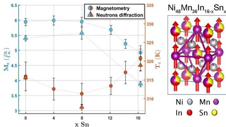
Figure 1: On the left: dependence of the saturation magnetization and Curie temperature versus the Sn at.% content. On the right: sketch of the magnetic and nuclear structures of  $\text{Ni}_{48}\text{Mn}_{36}\text{In}_{16-x}\text{Sn}_x$ .
