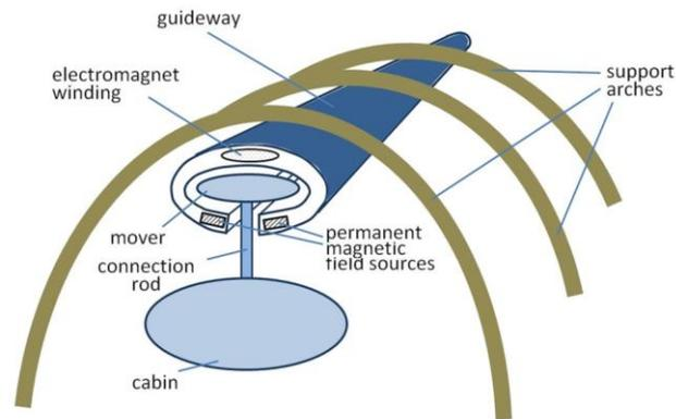
Figure 1: Magnetolevitation system based on arch-type trestle with lower cockpit location.
