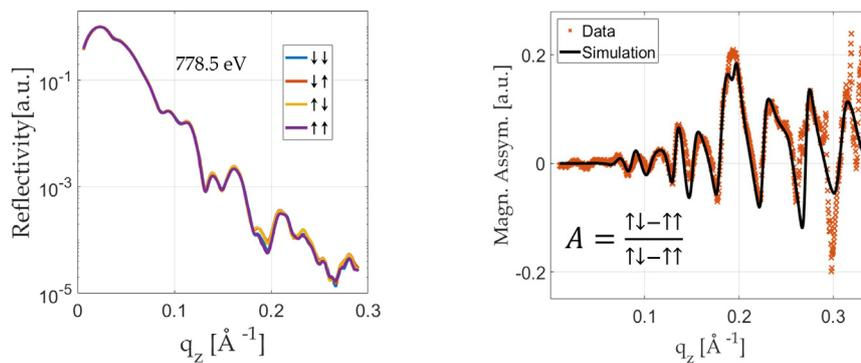
Figure 1: left: Resonant reflectivity curves measured at 778.5 eV (Co L<sub>3</sub> edge) with parallel (blue and purple) and antiparallel (orange and yellow) alignment of x-ray polarization and magnetization. right: Measured and with ReMagX [3-5] simulated magnetic asymmetry A at 778.5 eV (Co L<sub>3</sub> edge).
