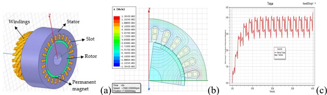
Figure 1: The BLDC motor structure(a), B analysis results (b) the torque versus time graph(c).
