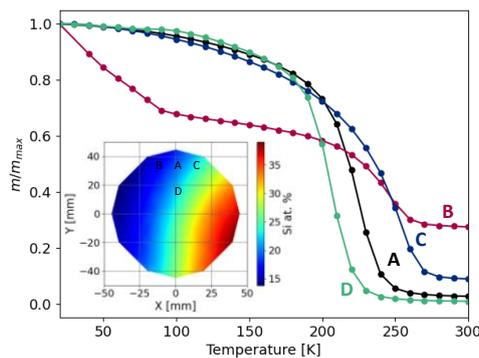
Figure 1:  $M(T)$  measured in-plane under an applied field of 50 mT, as a function of position of a La-Fe-Si film of nominal thickness 5  $\mu\text{m}$ , annealed at 900°C for 5 minutes. Inset: Si composition map of the same film in the as-deposited state.
