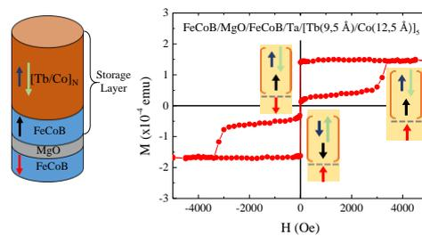
Figure 1: Left: Schematic of the AOS-MTJ. Right:  $M(H)$  of the AOS-MTJ including the optically switchable electrodes and the FeCoB sensing layer.
