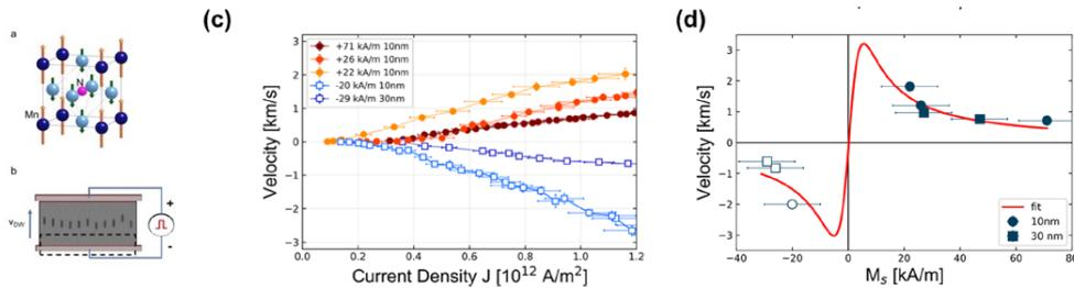
Figure 1: (a) anti-perovskite structure of Mn<sub>4</sub>N; (b) differential Kerr images showing the DW displacement in 1 $\mu$ m-wide strips under the application of current pulses; (c) DW speed vs. current density for Mn<sub>4-x</sub>Ni<sub>x</sub>N films with different Ni content, below and above the magnetisation compensation point; (d) fit to the  $q$ - $\phi$  model.
