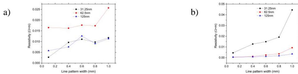
Figure 1: Resistivity of a)  $\text{Co}_{67}\text{Fe}_4\text{Mo}_1\text{Si}_{17}\text{B}_{11}/\text{Au}/\text{Co}_{67}\text{Fe}_4\text{Mo}_1\text{Si}_{17}\text{B}_{11}$  and b)  $\text{Co}_{67}\text{Fe}_4\text{Mo}_1\text{Si}_{17}\text{B}_{11}/\text{Au}/\text{Ni}$  vs line patterns width for three different thickness  $\text{Co}_{67}\text{Fe}_4\text{Mo}_1\text{Si}_{17}\text{B}_{11}$  film on substrate.
