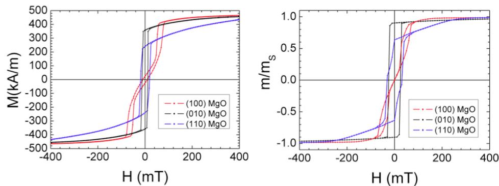
Figure 1: Experimental (left) and simulated (right) hysteresis curves, obtained applying a magnetic field along different directions of the MgO substrate.
