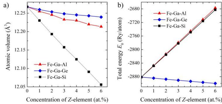
Figure 1: (a) The calculated atomic volume and (b) total energy for D0<sub>3</sub> structure of Fe Fe<sub>75</sub>Ga<sub>25-x</sub>Z<sub>x</sub> alloys depending on Z concentration (at.%).
