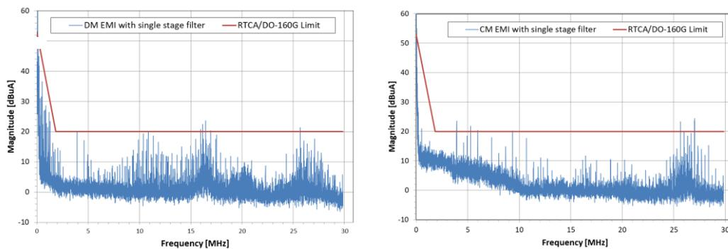
Fig. 2: CM and DM EMI with the single stage filter used for an actuator for avionic environment.
