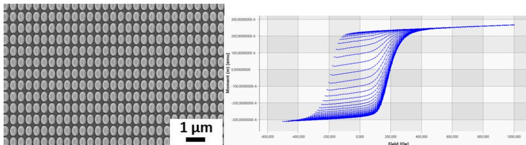
Figure 1: Left: Scanning electron microscopy image of a nano-imprinted array of elliptical cylinders of size 400nm x 200nm. The total number of ellipses is more than  $10^8$  on  $1 \text{ cm}^2$ . Right: Example of FORC measurement of this array with 40 nm thick CoFeB.
