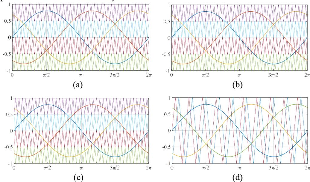
Fig.1: PWM multicarrier modulation schemes with sinusoidal reference: (a) Phase Disposition - PD; (b) Phase Opposition Disposition –POD; (c) Alternative Phase Opposition Disposition –APOD; and (d) Phase Shifted – PS.
