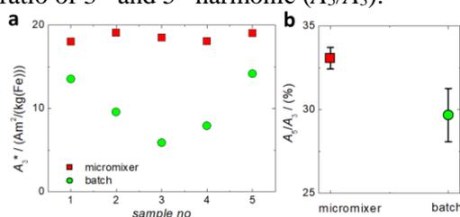
**Figure:** Dynamic magnetic susceptibility of MNP samples from two different synthesis approaches: **a:** Variation of 3<sup>rd</sup> harmonic amplitude of five MNP samples synthesized by micromixer (red squares) and conventional batch (green) procedure. **b:** Mean and standard deviation of the corresponding MPS spectra for micromixer and batch synthesized samples.
