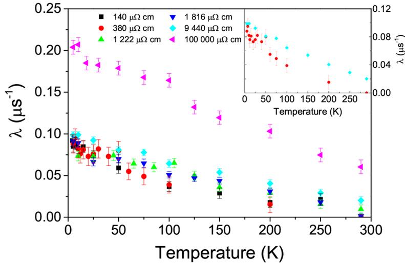
Figure 1: Temperature dependence of the muon spin relaxation rate of electronic origin for all samples in this work.
