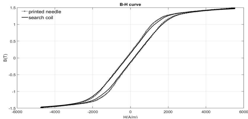
Figure 1: hysteresis loop when using printed needle and search coil.
