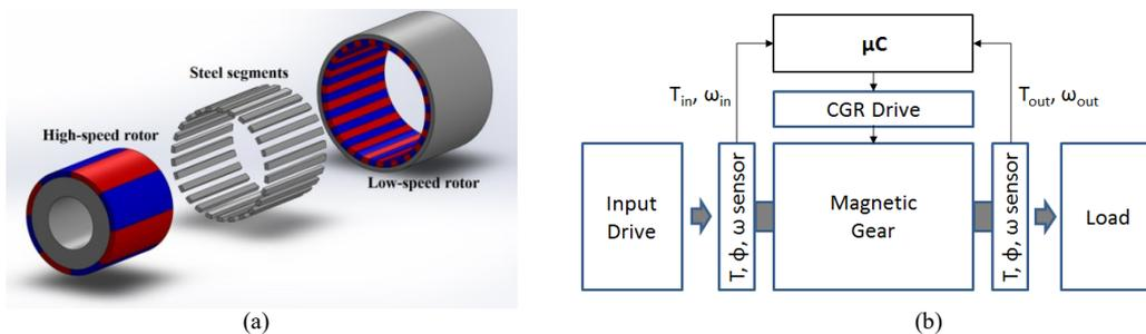
Figure 1: CMG assembly (a), and control system block diagram (b).
