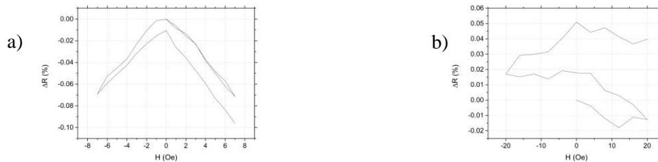
Figure 2: Magnetoresistance of a)  $\text{Co}_{67}\text{Fe}_4\text{Mo}_1\text{Si}_{17}\text{B}_{11}/\text{Au}/\text{Co}_{67}\text{Fe}_4\text{Mo}_1\text{Si}_{17}\text{B}_{11}$  and b)  $\text{Co}_{67}\text{Fe}_4\text{Mo}_1\text{Si}_{17}\text{B}_{11}/\text{Au}/\text{Ni}$  at 0.4 mm line width for perpendicular H (Oe) & I (A).
