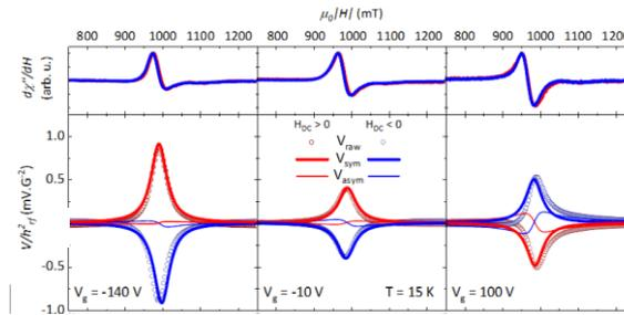
Figure 1: *FMR curves (top) and spin signals (bottom) for different values of the gate voltage in a STO-based 2DEG, for a positive (red) and negative (blue) applied DC magnetic field.*
