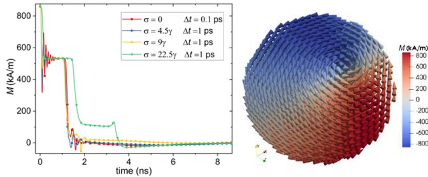
Figure 1: Left: Time evolution from saturation to remanence state of the radial component of the magnetization of a 100 nm permalloy nanosphere, showing the effect of  $\sigma$ . Right: Remanent state of the sphere; the cones represent the magnetization vector direction.
