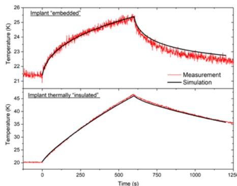
Figure 1 – Experimental validation of the computational tool.
