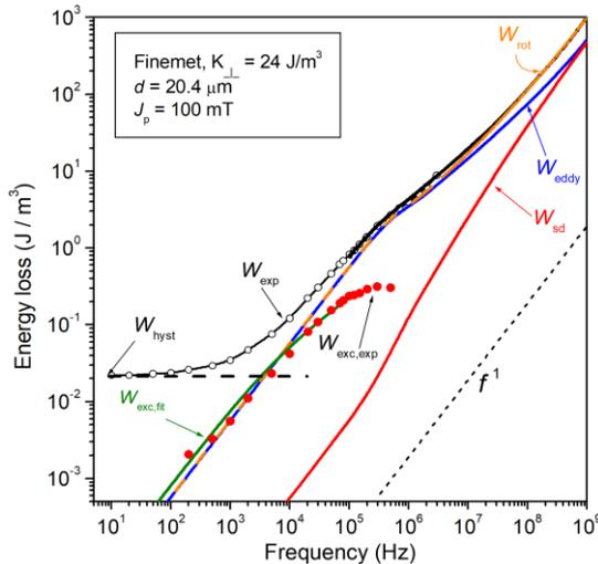
Figure 1: DC-1 GHz energy loss  $W(f)$  in a nanocrystalline ribbon with transverse anisotropy  $K_{\perp} = 24 \text{ J/m}^3$ . Once the quasi-static loss  $W_{\text{hyst}} = \lim_{f \rightarrow 0} W(f)$  is identified, the rotational contribution  $W_{\text{rot}}(f)$ , the sum of eddy current  $W_{\text{eddy}}(f)$  and spin damping  $W_{\text{sd}}(f)$  terms, and the domain wall related dynamic loss contribution  $W_{\text{exc}}(f)$  are obtained.
