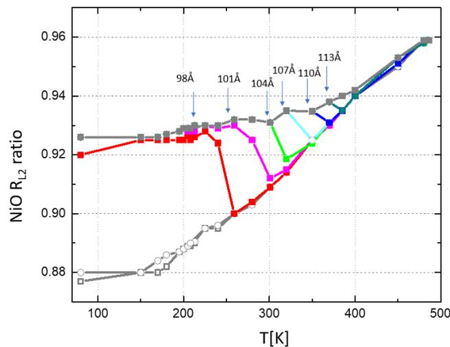
Figure 1: Temperature dependence of XMLD, defined here as  $R_{L2}$  ratio of two absorption peaks of NiO at the L2 edge. Possibility to tune the critical temperature of AFM spins switching is demonstrated.
