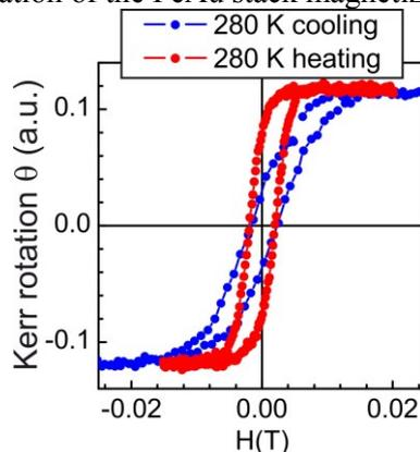
Fig. 1. The PMOKE loops collected at 280 K during cooling and heating process.
