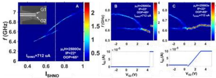
Figure 1. (A) Frequency vs. SHNO current profile. The inset shows were to top electrodes are located. Effect of memristor voltage ( $V_G$ ) sweep on power spectral density for forward (-3 to +4.5 V) and (C) backward (+4.5 to -3 V) sweeps.
